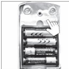
1. Loosen the battery cover screw, open the cover and put in the batteries.
