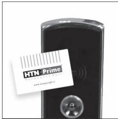
1. Touch the card reading area, you will see the password screen light on and hear the beep sound, then open the door with master card.
