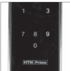
3. Press "7" key (delete the card) or "9" key (delete the password) to enter into the operation window from the system, after hearing the beep sound, input the double-digit code of card or password which are delete-waiting (such as 1-3), and press "#" key to confirm the deletion, when you hear "didi", it indicates the successful deletion.
